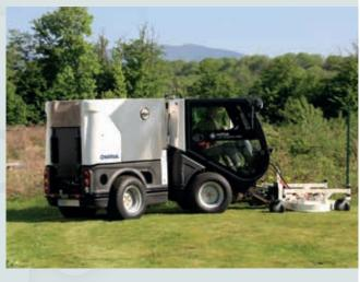
The City Ranger 3500 can be equipped with green quality attachments like rotary mowers for grass collecting, supplying a cutting width of up to 1.500 mm with an adjustable cutting-height of 30 to 150 mm.
