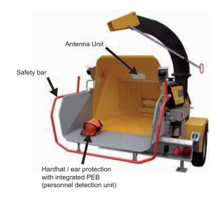
When entering the electromagnetic field generated by the sending / receiving unit, the feed rollers are instantly stopped
