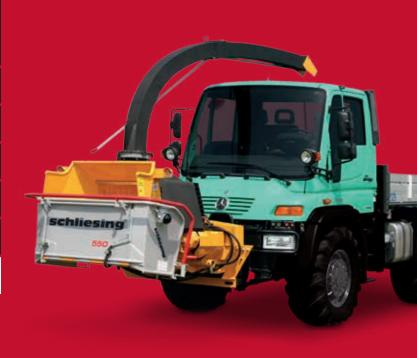
schliesing wood chippers comply with the safety regulations of DIN EN 13525.
