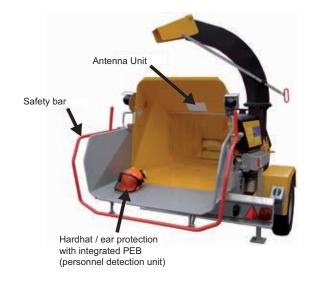
When entering the electromagnetic field generated by the sending / receiving unit, the feed rollers are instantly stopped
